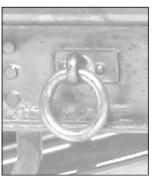
4. Emboss bolt heads and fold up the headstocks (parts 4). Solder coupling plates (parts 5) over the coupling slots but ensure that the slot remains free from solder.
